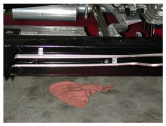
2. First remove both gas line clips. Thread holes using a 5/16"-28 tap. Use 4 clips and 2 bolts supplied to mount fuel lines. The 5/16" line goes on top. The 3/8" line goes on the bottom. Note position of lines on rear clip. Picture #1. Do not mount brake line at this time.
