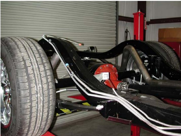
7. Attach 3/8" stainless steel hose to 3/8" line at frame. Attach other end with 45 degree fitting to fuel supply log on engine. Pictures #5 and #6.
