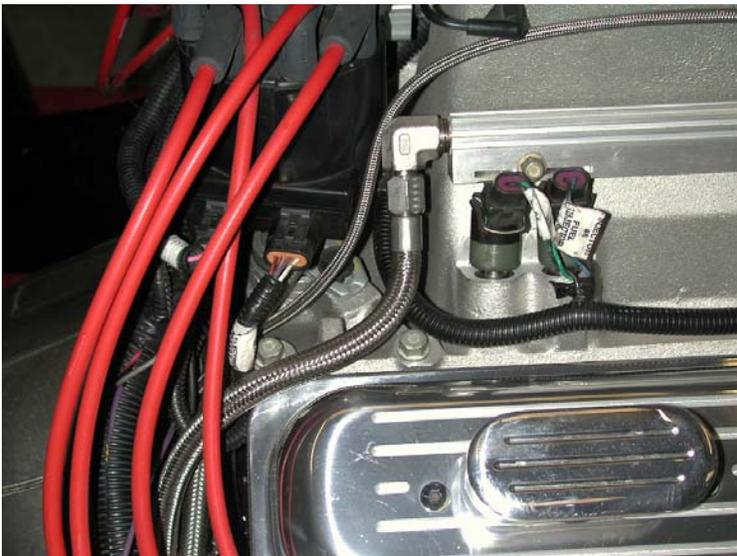
8. Attach return 5/16" stainless steel braided hose to fuel line at frame. Attach other end to regulator at driver's side of the engine.
