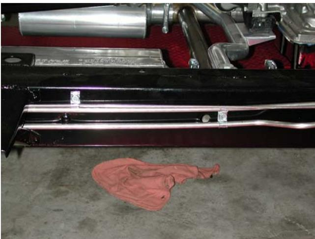
2. First remove both gas line clips. Thread holes using a 5/16"-28 tap. Use 4 clips and 2 bolts supplied to mount fuel lines. The 5/16" line goes on top. The 3/8" line goes on the bottom. Note position of lines on rear clip. Picture #1. Do not mount brake line at this time.
