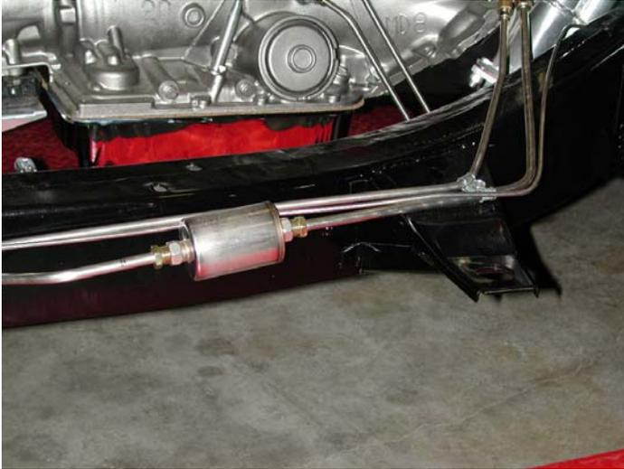
5. Attach brake line at this time. Run brake line over the top of the 5/16" return line using supplied clips and bolts. You will have to drill new holes to attach this line. Picture #2.
